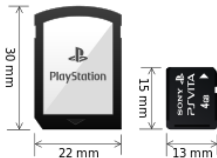
Figure 2. PSVita External Media - Left: The Vita Card, Right: Vita Memory Card
