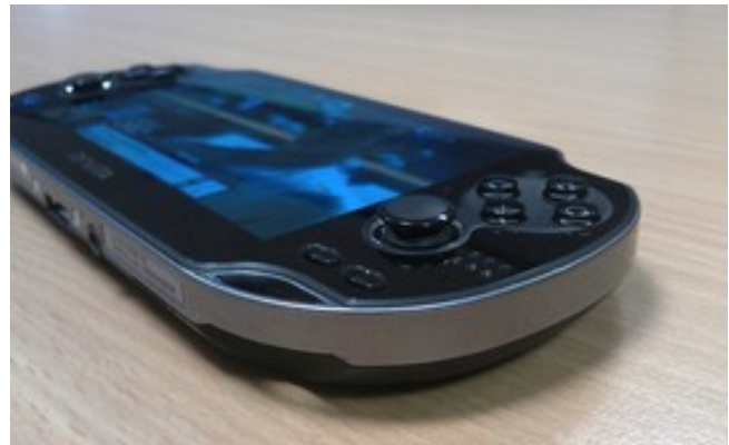
Figure 1. PSVita Development Kit - Sony PlayStation Vita Development Kit PDEL-1001 - What is so good about a PSVita DevKit over a PSVita Debug/Test console? For one thing, you can debug code as if you were running it on your PC, furthermore, you can dump/debug the PSVita kernel information.
